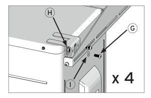
FASTEN SIDE PANELS (D & E) TO BRACKETS (C) WITH PARTS (G, H, & I) X8
