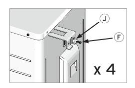
ATTACH 4X BRACKETS (C) WITH THE HARDWARE YOU JUST REMOVED.
