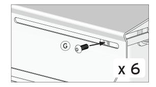
ATTACH ASSEMBLED COVER ONTO SIDE PANELS (D & E) WITH BOLT (G) X 6. DON'T FASTEN TOO TIGHTLY.
