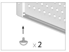
SCREW FOOTER HARDWARE (E) INTO THREADS ON PART (A).
