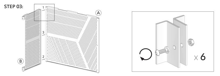
FASTEN HARDWARE (F-H) TO CONNECT PARTS (A & B). KEEP TABS FACING UPWARD. REPEAT FOR PART (C). LOOSELY THREAD ALL HARDWARE BEFORE TIGHTENING.
