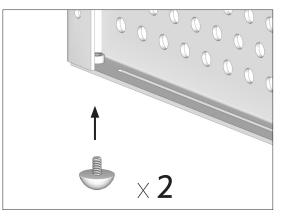
SCREW FOOTER HARDWARE (E) INTO THREADS ON PART (B). REPEAT STEP FOR PART (C).
